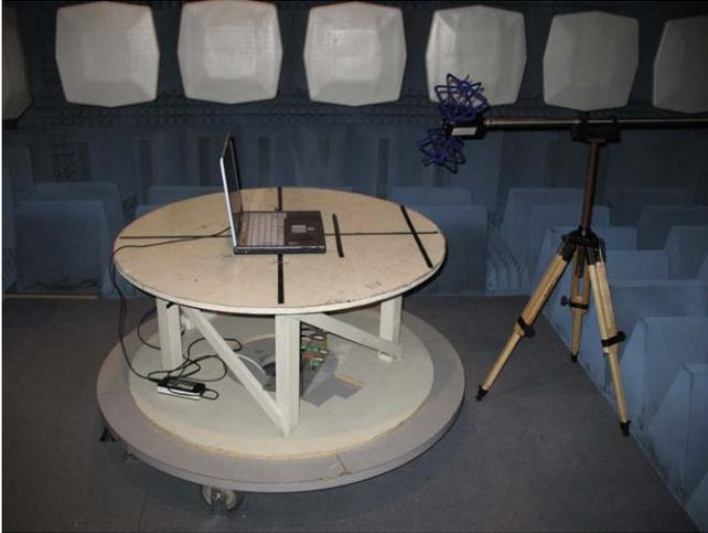
Fig. 1. Reference emission measurement setup inside the shielded room of EWC laboratory.
