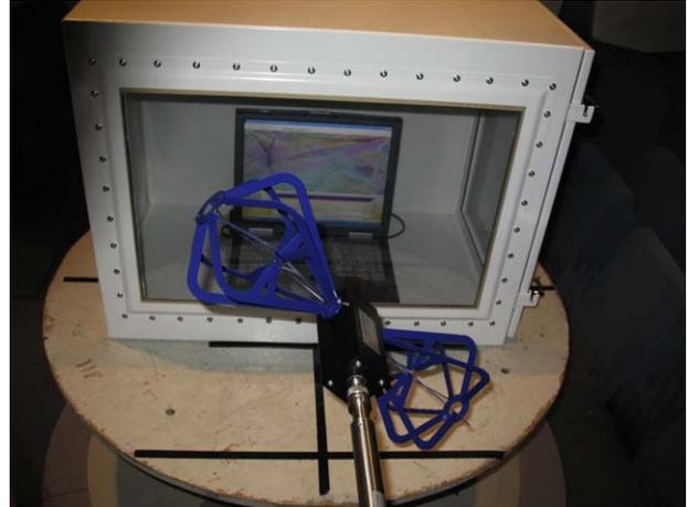
Fig. 2. The laptop inside the shielding cabinet.
