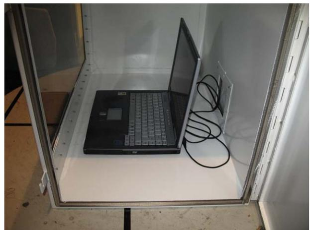
Fig. 3. A view into the open shielding cabinet with the cable access panel visible behind the laptop.
