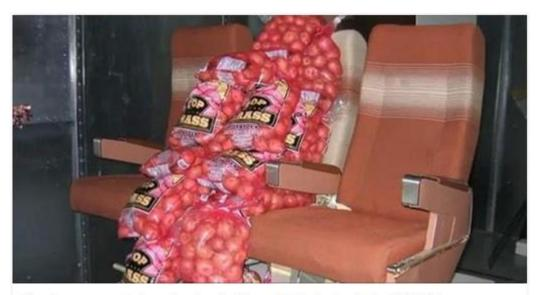
Boeing uses potatoes instead of people to test wi-fi - BBC News US aircraft manufacturer Boeing used unusual substitutes for passengers while testing its in-flight ...
